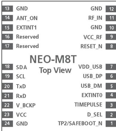
Figure 3: NEO-M8T Pin Assignment
