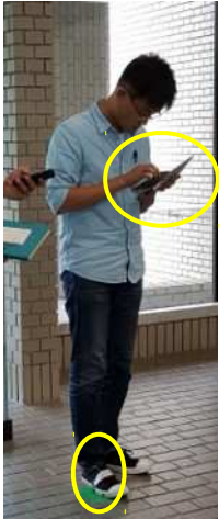
Foot-mounted IMU & Laptop
