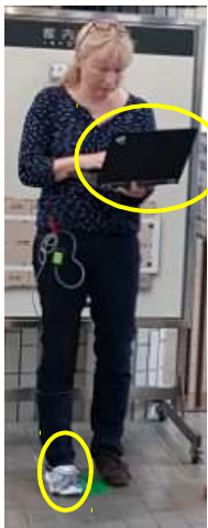
Foot-Mounted IMU & Laptop
