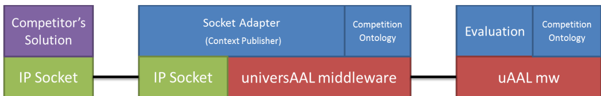
Figure 1 Router-like architecture of the SocketAdapter solution
