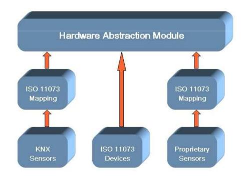
All connected systems are mapped to 11073 standard, e.g. KNX, LON, and other proprietary protocols (Eaton, Legrand,...)
