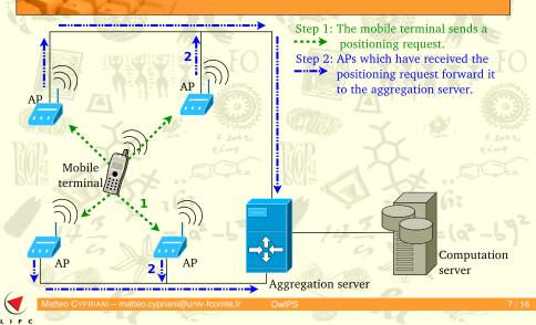
Step 1: The mobile terminal sends a positioning request. Step 2: APs which have received the positioning request forward it AP to the aggregation server. AP Step 3: The aggregation server aggregates the received information and forwards it to the computation server. Mobile terminal Computation AP AP server Aggregation server
