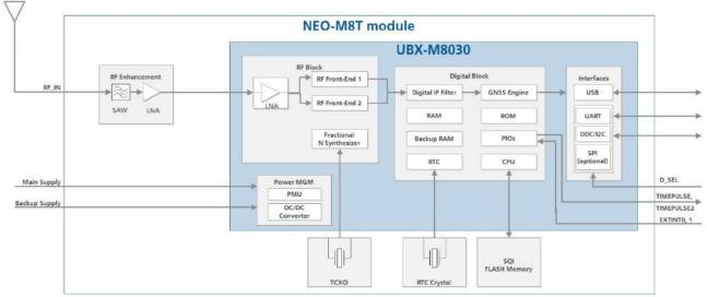
Figure 1: NEO-M8T block diagram
