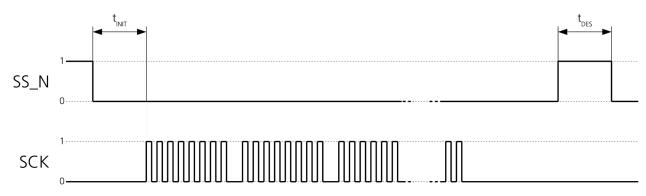
Figure 5: SPI timing diagram
