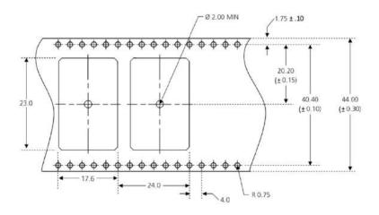
Figure 9: Dimensions and orientation for LEA-M8T modules on tape
